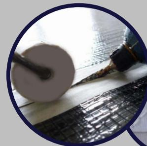
Anti-chafe 3 step stitched seams or we offer an upgrade of a fully bonded seams option for the ultimate low stretch sail
