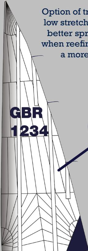
Option of tri-radial using a very low stretch material is used for better spreading of the loads when reefing, better furling and a more efficient shape.
