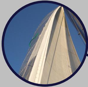
Spectra or anti-tortion rope luff to support the loose luff and enable the use of a furler
