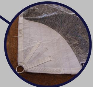
Clew corner reinforcement - radial patches
