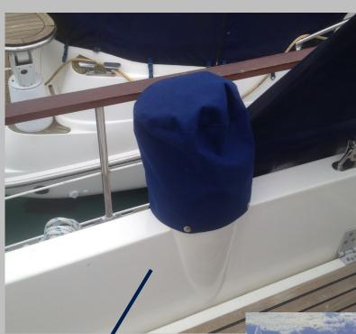
We use anti-wick thread which swells up when wet to make the cover water proof or an option to upgrade of thread to 'Tenara', guaranteed for 15 years, almost impervious to UV degradation so perfect for use in high UV areas, acid rain and other pollutants, however 'Tenara' is not an anti-wick thread so it can leak in big downpours.
