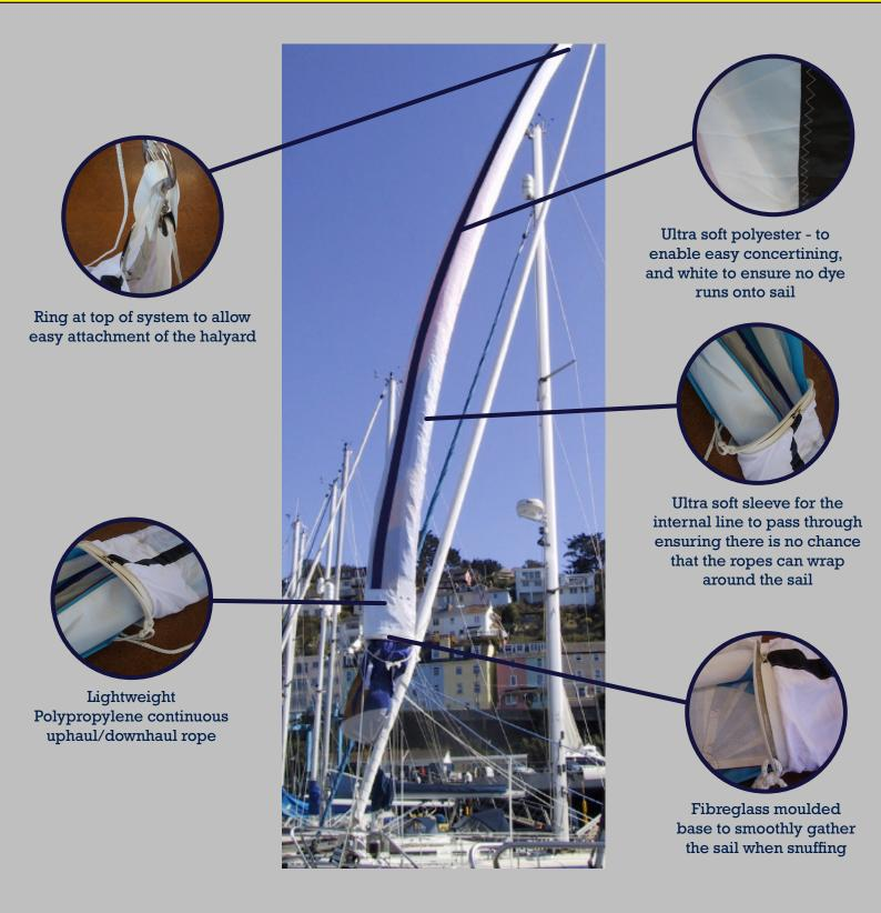
The Snuffer is an essential addition to downwind sail on a short handed Cruising or Offshore Racing yacht. The snuffer allows the spinnaker or cruising chute to be hoisted whilst contained in a polyester tube. When the tack and sheets are attached and the sail is hoisted - bear away onto a broad reach with the snuffed sail in the lee
