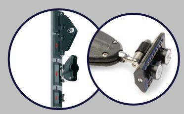
RONSTAN BALLSLIDES – Recirculating Ball bearing cars that bear on the aft face of the mast for almost minimal friction. Formally known as Frederiksen slides these are the very lowest friction without requiring a separate track. As the slides fit into the existing mast groove just batten slides or battens and head car can be opted rather than having to buy intermediate slides as well. Series 6 for boats up to about 40ft while series 8 for boats up to around 60ft.
