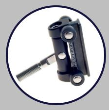
RUTGERSON BATTCAR – Self lubricating low friction composite slides. Excellent Value and the most popular batten car option on the market. Features 4 wheels that bear on the aft face of the mast to reduce compression friction and reduce any rocking in the mast. Standard versions suitable for boats up to 40ft with high load options suitable up to 60ft boats.
